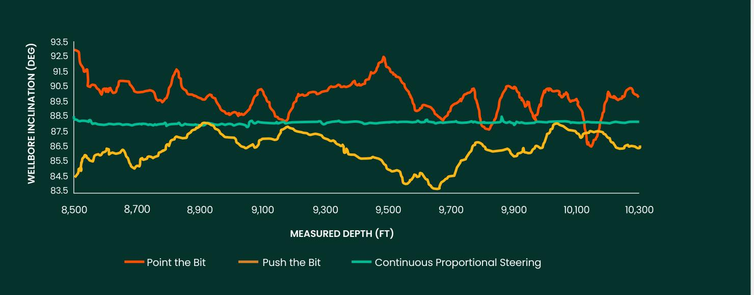
Comparison of well tortuosity from the study using high resolution wireline surveys from three offset wells. The difference is unmistakable when comparing wells drilled with push-the-bit (yellow), point-the-bit (orange), and continuous proportional steering (green) technologies. The AutoTrak RSS clearly delivers substantially superior hole quality.
