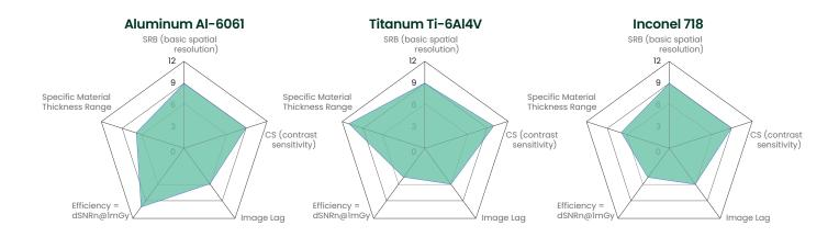
The Dynamic 41|200p+ detector characterization according to ASTM E2597-14 for AL, TI and Inconel is displayed below (valid for specific detector gain settings):
