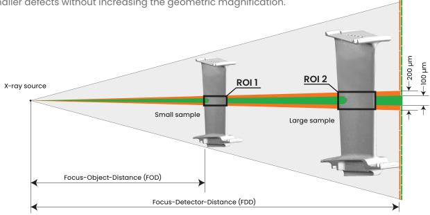
Scan resolution of ROI 1 is equivalent to ROI 2, but ROI 2 is 8 times larger due to smaller pixel allowing scanning larger parts with smaller magnification.
