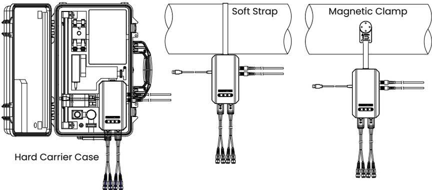
Figure 6: PT900 Transmitter Mounting Options
