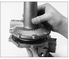
Figure 34 Placing Spring Housing onto Pilot Body
