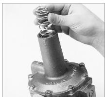
Figure 35 Installing the Spring into the Spring Case
