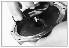
Make sure lever is centered in the diaphragm retainer
