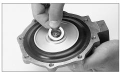
Figure 33 Place one Spring Washer on the Diaphragm assembly
