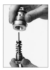
Figure 22 Insert the assembly into the Body Insert - the orifice should "snap" into place
