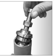
Figure 16 Installing the closing cap assembly for Pilot with the Red, Plated, Blue, and Purple Springs 6B. PILOTS WITH BLACK AND GREEN SPRING: Install Closing Cap with Adjusting Screw, Spacer, Sealing Nut, and O-Ring. The spacer prevents the Black and Green springs from being over compressed.
