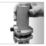
Figure 14 Placing the Spring Housing on the Pilot Body
