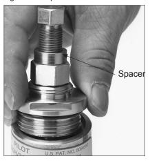
Figure 17 Installing the closing cap assembly with spacer (to prevent spring over compression) for Pilots with the Black and Green Springs
