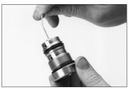
Figure 11 The orifice can be pushed out of the Body Insert (Cartridge) using a paper clip
