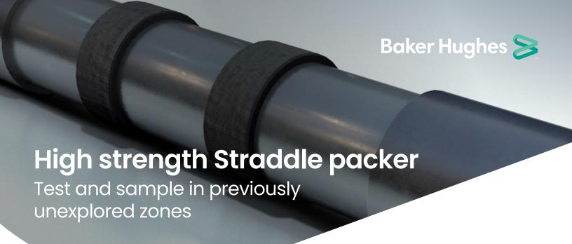
The high strength Straddle packer module is an additional component of the Baker Hughes fluid characterization and testing portfolio. It features two custom-designed inflatable packer elements that are configured to isolate a 1-meter zone of the borehole to enable various tests to be conducted in this isolated interval. Full combinability with all Reservoir Characterization explorer™ (RCX™) service modules build on the proven reliability of the RCX platform.
