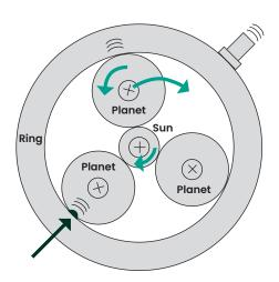
Figure 1. Planetary gear arrangement showing debris that causes a detectable impulse vibration.
