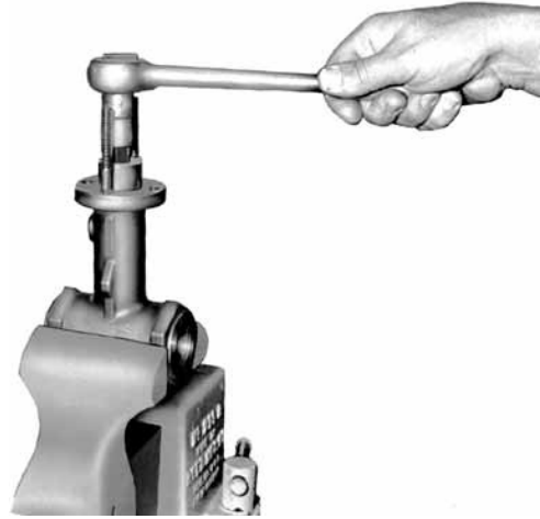
Figure 19 - Tightening the seat-ring retainer (4)
