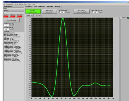
The location of the peak on the X-axis confirms the identity of water. The y-axis is related to the partial pressure of water and therefore the concentration. The system is equipped with AuroraView software, which enables users to capture the absorption spectrum and export it to other application programs such as Excel™.
