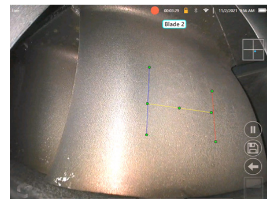
Fig 9c. Blade Counter active showing original tracking region
