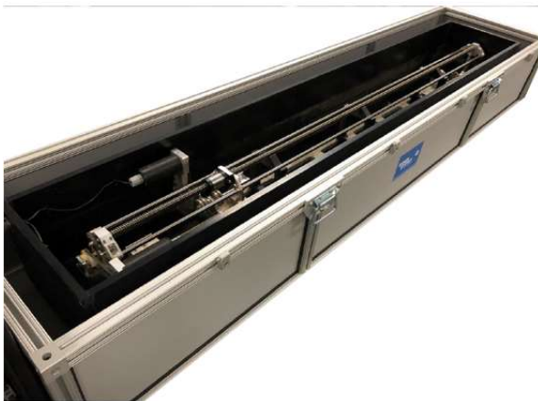
Figure 2: Prototype Tube inspection system – self-contained water tight inner shell within outer transport case.
