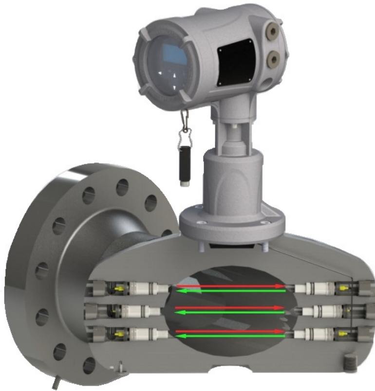
Figure 1: Transducer Paths Across Flow Direction
