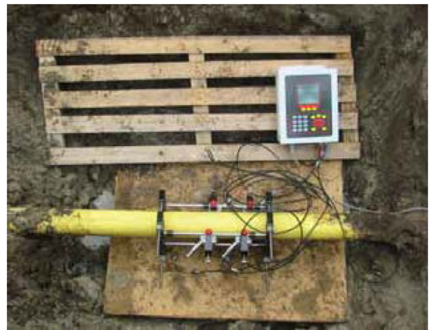
C-RL transducers installed on a 4 in (100 mm) carbon steel pipe with a 0.08 in (2mm) PE coating (outside)
