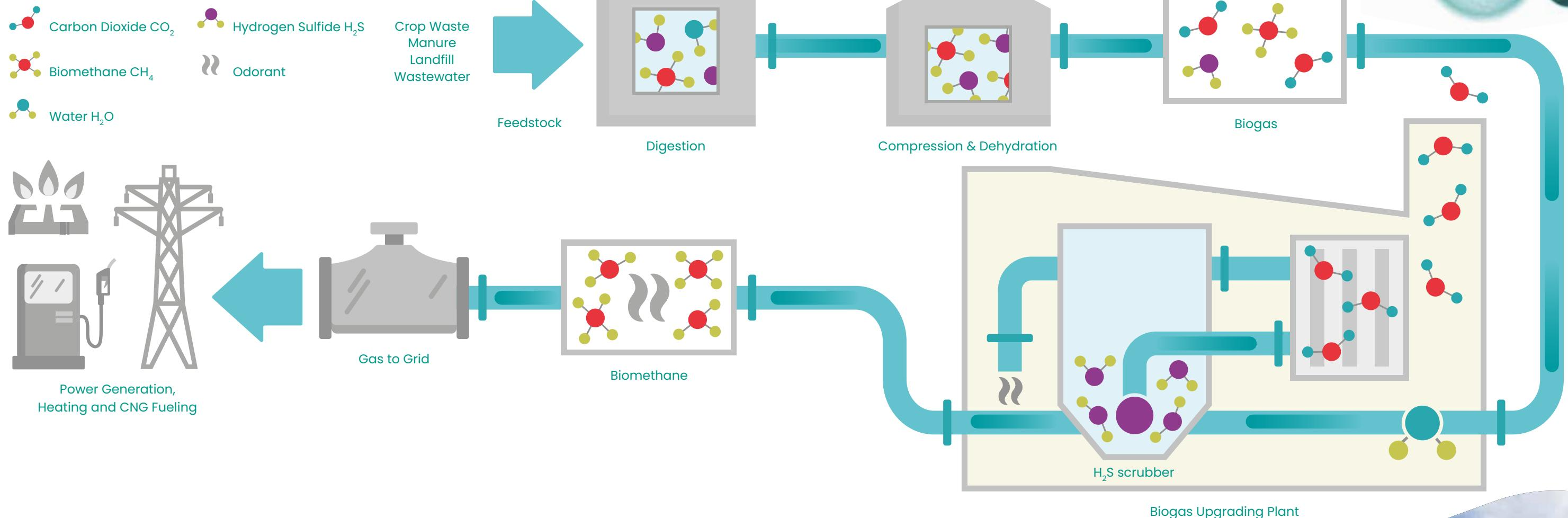
Biogas is increasingly seen as a more renewable source of natural gas. Biogas is the mixture of gases produced by organic waste in the absence of oxygen. Upgrading biogas to biomethane includes removing carbon dioxide and water vapor along with trace gases such as nitrogen, hydrogen sulfide, and hydrogen.
