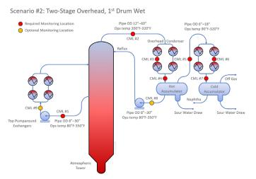
Scenario 2 – Proposed Rightrax Sensor Locations Two-Stage Overhead/1st Drum Wet
