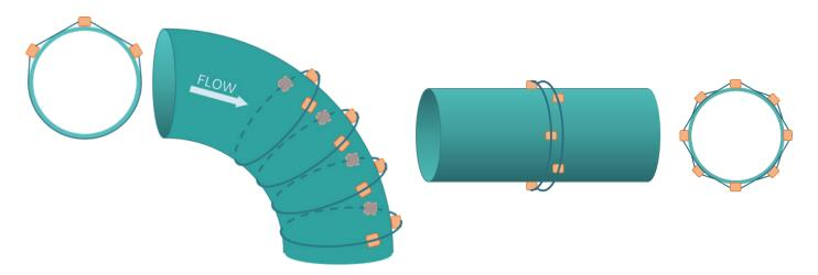
Figure 1: Sensor configuration on elbows
