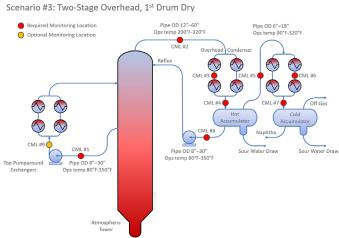
Scenario 3 – Proposed Rightrax Sensor Locations Two-Stage Overhead/1st Drum Dry
