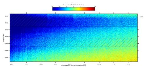
SureVIEW Coil post-stimulation DTS results show warmback temperature changes, aiding in the identification and optimization of acid and diverter placement.
