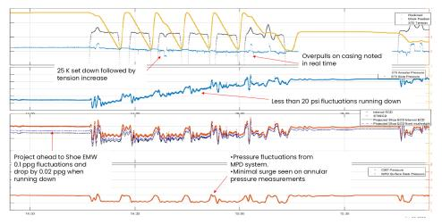
Detailed view of running the screens in the openhole section. Real-time monitoring of the set-down weights directly above the screens showed the initial inertia of the string as weight was transferred down followed by the actual movement of the screens downhole.
