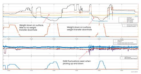
The first attempt to set the openhole screens was made with weight set down at the surface, but with minimum to no weight transferred down to the packer. The packer was not set, as confirmed by the bore and annulus pressures. A subsequent set down showed the weight transfer occurring and a successful setting of the packer.
