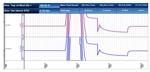
Real-time fluid level results transmitted during the TCP operation. The annular pressure measurements were converted to a fluid level using known volumetrics. The large increase is the pressure used to charge the guns. The sharp drop off is the drop in fluid level when the guns fired, then showing the losses over time due to the overbalance. After observing the rate of loss over time the well was balanced and put on the trip tank for additional monitoring.
