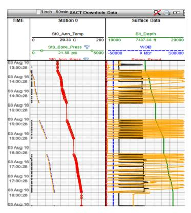
Since the XACT telemetry service is fullbore through and does not require fluid or flow to transmit, it is possible to send data while tripping. Work string and annular pressures were transmitted every 20 seconds throughout the entire operation. This allowed continuous monitoring of the well, even while tripping out of the hole.
