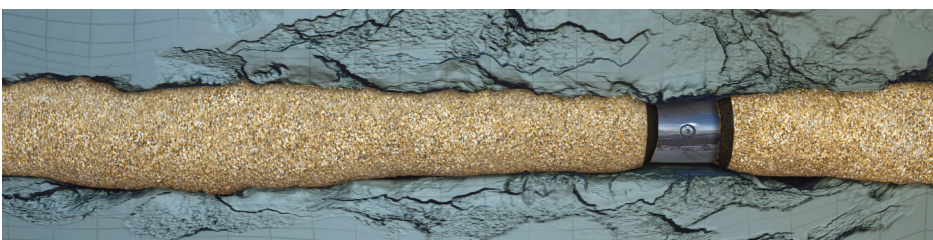
The SMP media is run in hole in a compressed state with an OD smaller than the wellbore (top). When activated, the SMP material expands and fills the entire annulus, applying residual stress to the sandface while acting as a filtration medium (bottom).
