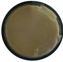
Oil-based mud filter cake before treatment with MICRO-WASH<sup>™</sup> treatment.
