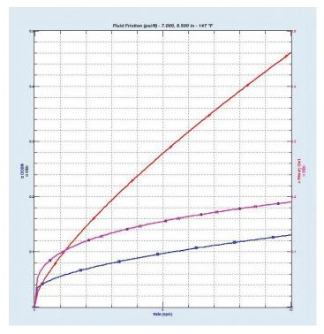
Fluid friction chart showing rheological hierarchy between mud, spacer, and cement.
