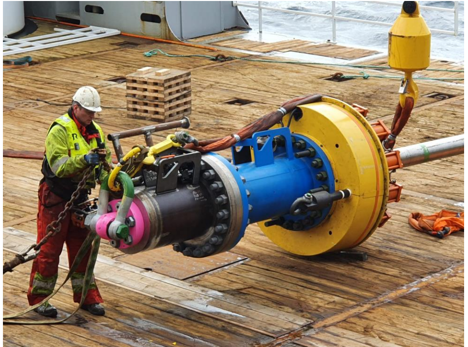
The Terminator cutting system only requires 100 hp and virtually no deck spread space, delivering a simple, environmentally-sound solution for subsea wellhead removal at any water depth.
