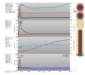
An operator in south India was facing production issues in an exploratory gas well. The company was trying to evaluate the producability of the formation which had near-wellbore formation damage from drilling, completions, and perforating activities. In addition, the low native permeability of the formation (10% porosity and 1-4 mD permeability) had led to greater formation loss and permeability in the damage zone.
