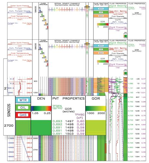
The IFX module provides a real-time interpretation of the contamination levels when sampling.
