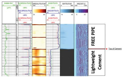
The Integrity eXplorer service showed a shear attenuation difference of ~50db/ft, confirming the presence and strength of the lightweight cement, while the CBL showed a compressive attenuation of only ~2 db/ft.
