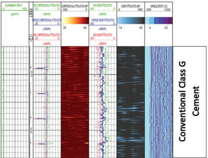
The CBL data agreed with the Integrity eXplorer service data in the upper section of the well containing conventional class G cement.
