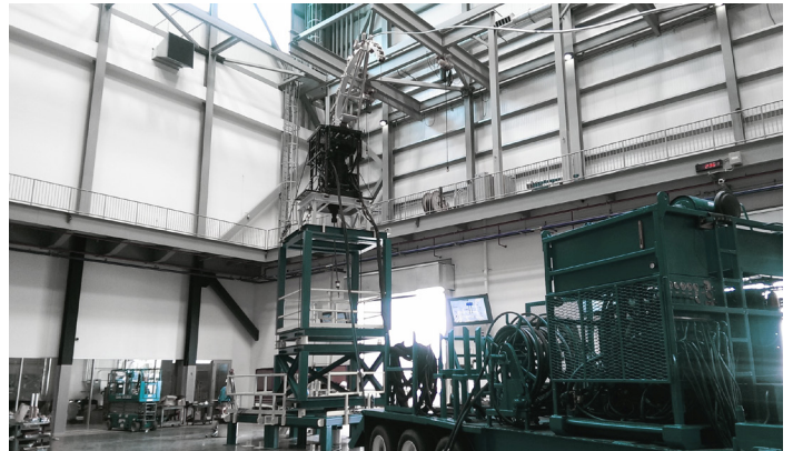
Figure 13: Coiled tubing unit and test well in the Baker Hughes Artificial Lift Research and Technology Center
