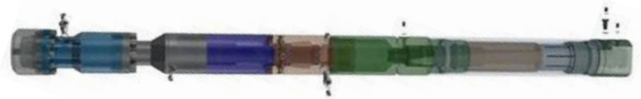
Figure 10: Electrical connection from the ESP motor to the power cable, with the shear sub shown in blue
