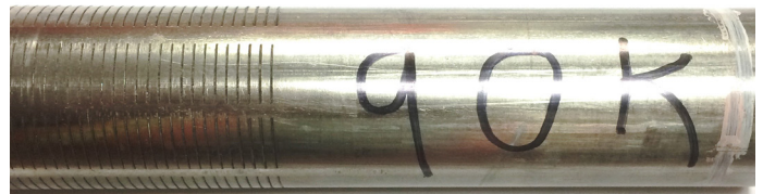
Figure 9: Actual test sample of coiled tubing loaded to 90,000 lb (40,823 kg)
