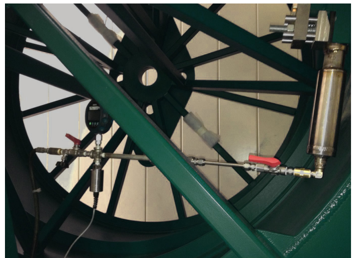
Figure 3: Pressure test setup for the power cable
