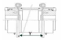
Model 13: single engagement coupling must NEVER BE USED ALONE, but always coupled to another model 13 to create a model 12.
